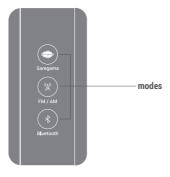
To choose a mode, press the corresponding mode button on the unit
